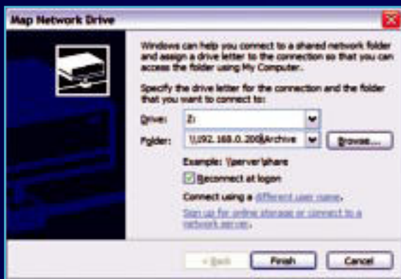
Mapping a static IP as a network drive makes accessing shared folders much easier.
